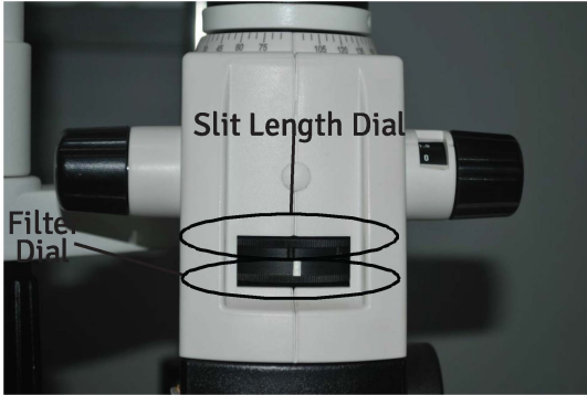
Figure-18 Filters and Slit Length
