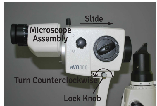
Figure -9 Install Microscope
