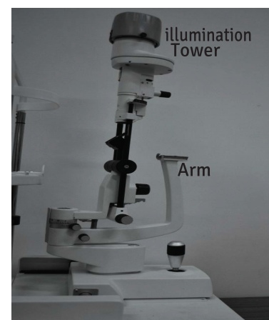
Figure. 6b Mounting Illumination Tower & Arm
