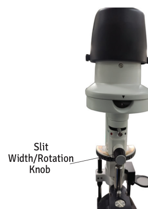
Figure-15 Adjust Slit Width
