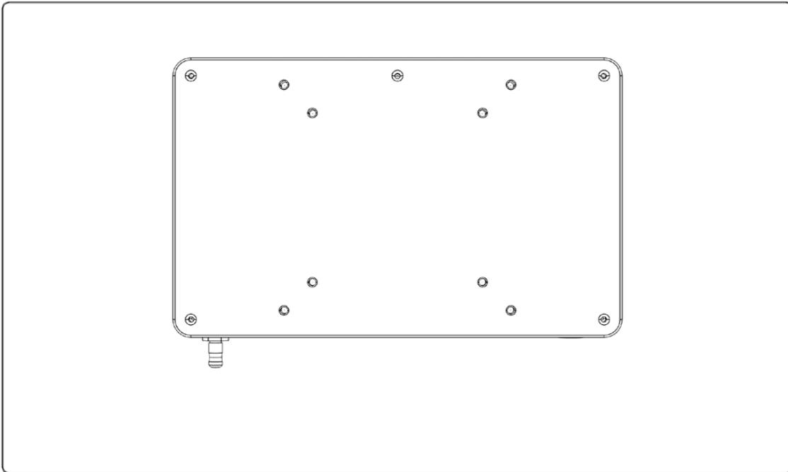
The back is VESA 75 and VESA 100 compatible and easily attaches to a matching monitor mount.
