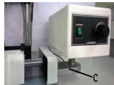
Figure- 7 Assembling Power Supply on the Power Supply Bracket
