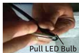
Figure 31a Changing Target Light LED
