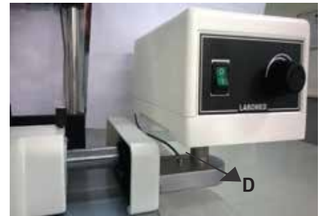
Figure.7 Assembling Power Supply on the Power Supply Bracket
