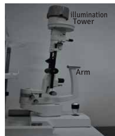
Figure. 6b Mounting Illumination Tower & Arm
