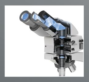
The highly streamlined Lx POL delivers reliability and comfort through user-friendly design and precision engineering. Tight design tolerances and the SF (Strain Free) optical system produce true polarization. A combination of an optical grade polarizer with high extinction properties, individually centerable POL objectives, and a perfectly matched analyzer provide outstanding contrast and clarity.
