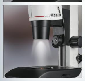
An ergonomic control cluster brings reflected and transmitted LED light controls within close proximity of macro zoom control, making it more intuitive for technicians to quickly switch back and forth without looking away from the eyepieces. Thus ensuring maximum efficiency.
